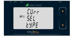
Pressing the " I Down" key will enter the "output 2 type edit" mode and scroll between voltage and current.
