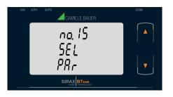
Pressing the " Down" key will enter into the "Parity & stop bit edit" mode and scroll the value between **odd:** parity with one stop bit
