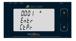
Pressing the " Down" key will enter the transducer into "CT Primary value edit" mode.
