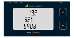
This screen allows the user to set Baud Rate of RS 485 port. The values displayed on screen are in kbaud.
