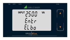
Pressing the " Down" key will enter into the "Input Elbow value edit" mode.
