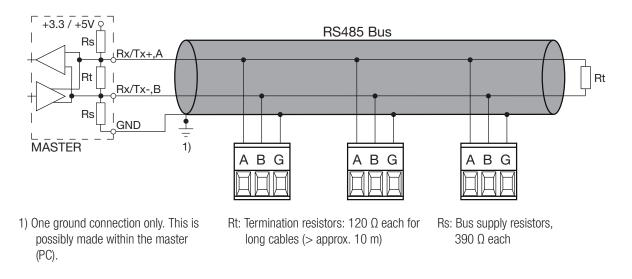
The signal wires (A, B) have to be twisted. G can be connected via a wire or via the cable screen. In disturbed environments shielded cables must be used. To avoid the possibility of loop currents, an Earth connection should be made at one point on the bus. Supply resistors (Rs) have to be present in bus master (PC) interface. Stubs should be avoided when connecting the devices. A pure daisy chain network is ideal.
